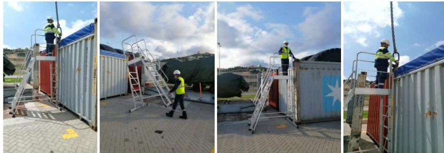
Flexible light weight Mobile Ladder Platform, used for OOGs, Special Handling preparations and container top check/repair – TM2
