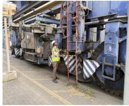
RTG Vertical Ladder Access Restriction Poke-yoke, when open Sensor is activated and RTG Gantry cannot be activated - PPV
