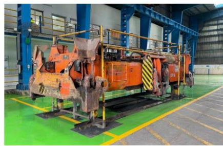
Spreader maintenance platform - External
